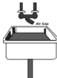
Air gap – a physical separation between potable water pipes and non-potable water sources
